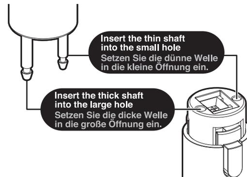
Insert the thin shaft into the small hole
