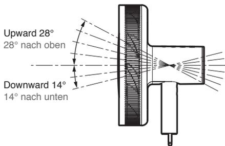
Vertical adjustments: 7 positions in 7° increments
