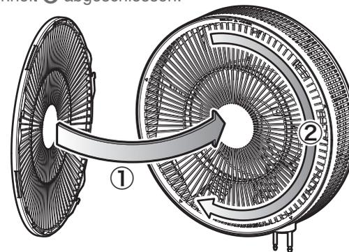
Turn the Front Guard **1** until the ▲ mark matches with the magnet on the Side Guard **3** to lock it in place.
