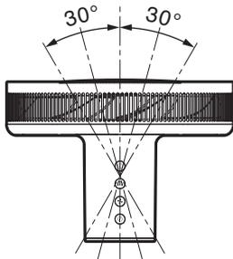
Horizontal adjustments: 5 positions in 15° increments
