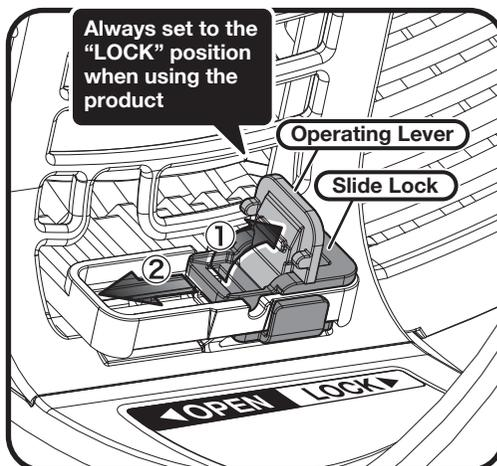
▲Slide the lock from the "LOCK" position to the "OPEN" position.
