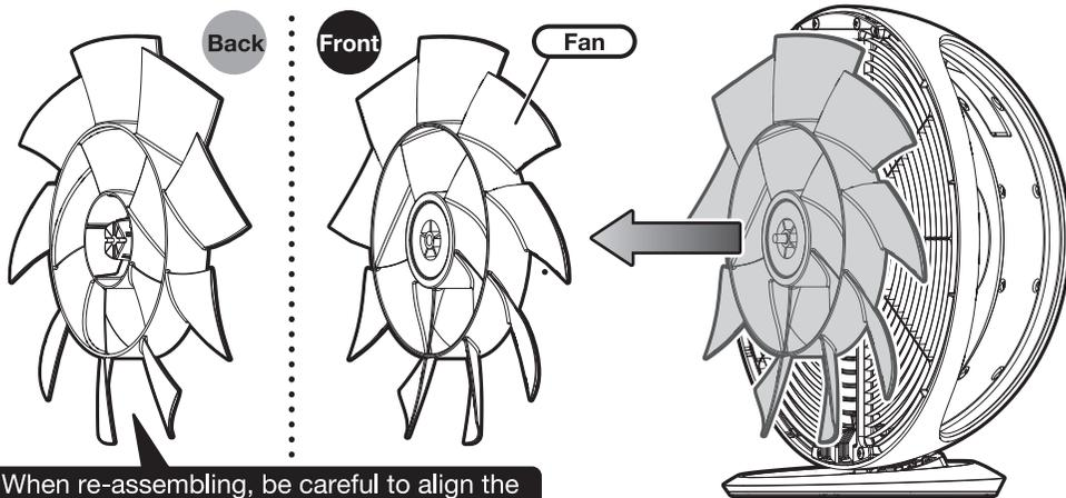
\* After maintenance is complete, re-assemble the parts in the order (4) to (1).
