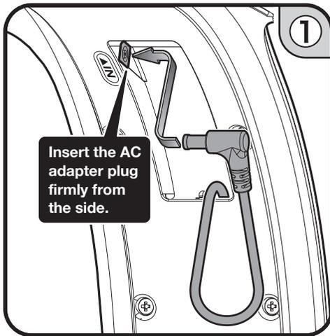
Insert the AC adapter plug firmly from the side.
