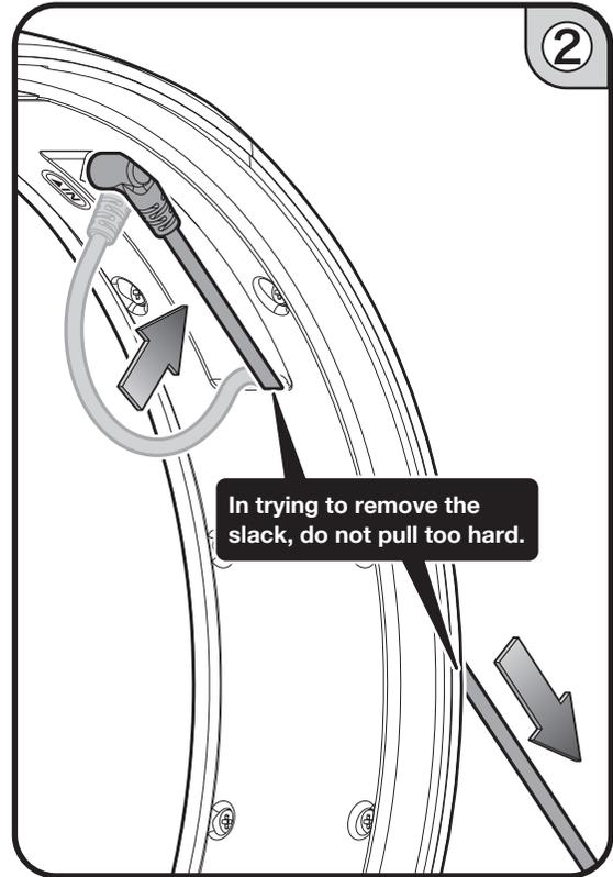
▲ Pull on the cord on the outside of the Body to remove the slack inside.
