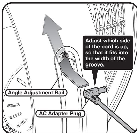
▲ Insert from the back of the Body deep into the uppermost part of the angle adjustment rail.
