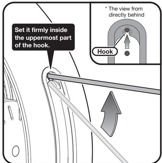
▲ Set it into the groove on the top of the angle adjustment rail and fix it firmly in place.
