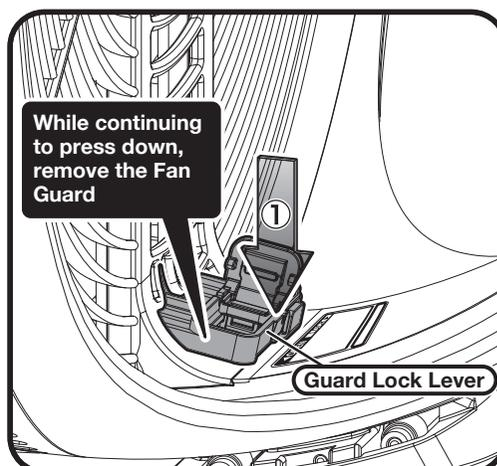
▲Remove the Fan Guard by disengaging it from the catch from beneath while the Guard Lock Lever remains depressed.
