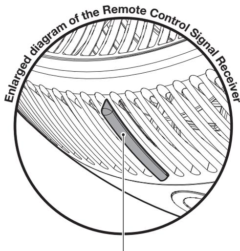
\* The transparent portion on the bottom of the front of the Fan Guard is the receiver for signals from the remote control.
