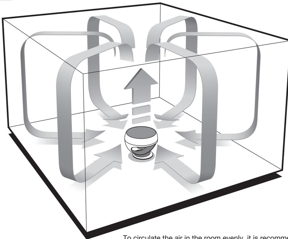
To circulate the air in the room evenly, it is recommended to **set up the device in the center of the space, with the fan aimed upward.**
